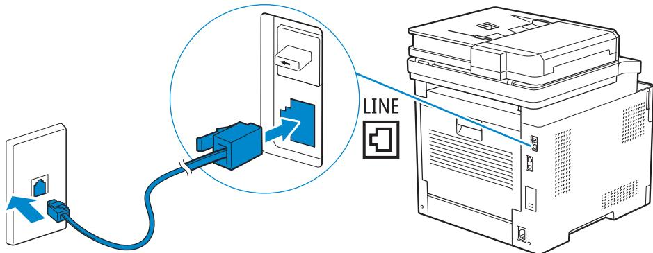
**NOTE:** If the phone communication is serial in your country (such as Germany, Sweden, Denmark, Austria, Belgium, Italy, France and Switzerland), and you are supplied with a yellow terminator, insert the yellow terminator into the phone connector.
